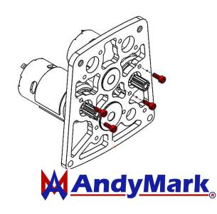
**Step 7**: Place Cluster Shaft for 2 Stage EVO Slim (am-3814) into the FR6ZZ bearing.
